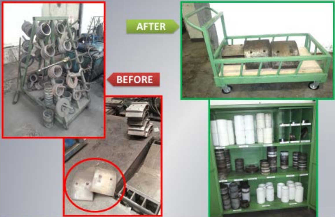
DESCRIPTION: RECONSTRUCTION OF STEEL STANDS TO STORAGE PUSH CARTS BENEFIT: TIME SAVING ON SETUP, VISUAL AND SAFETY IMPROVEMENT
